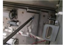
7. Disconnect the Connectors for Solenoids SOL3 & SOL4 from the header.
