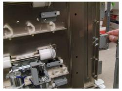
12. Carefully remove the Shaft.
