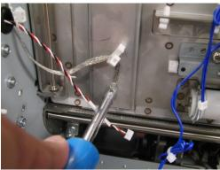
9. Remove the E-Ring from the bottom of the Idler Panel Shaft.
