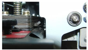
• Unlatch the acceleration idler panel and Entrance Idler panel to see the trail edge of the sheet. (the trail edge of the sheet will be skewed if one of the corners is jammed as opposed to the whole lead edge being jammed)
