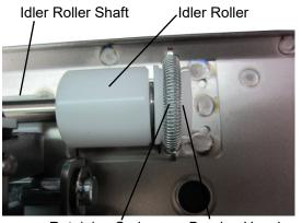
Retaining Spring Bearing Housing
