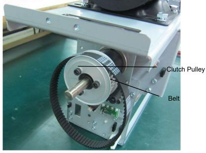
9. Place the new Belt around the Timing Pulley on the Punch Motor and the Clutch pulley.
