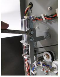
b. Insert a 0.25 to 0.5mm shim between the Diverter and the Lower Entrance Panel.
