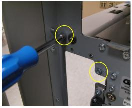
8. Remove the Screws (2) from the Rear Frame used to mount the Lower Exit Panel.
