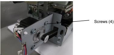
5. Adjust the belt tension such that there is a deflection of  $1\sim 2mm$ .
