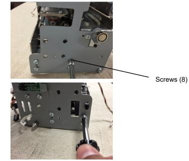
11. Remove the Steering Module from the Punch Module, by tilting the Steering Module as shown. This is to ensure the back side clears the self-clinching nut.
