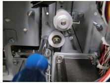
9. Remove (5) screws from the front frame that mount the Exit drive panel.
