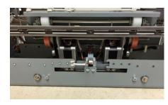
Note: There is no need to remove the Steering module if you have a screwdriver or a 5.5mm nut driver that will reach the (4) screws through the opening in the punch frame.
