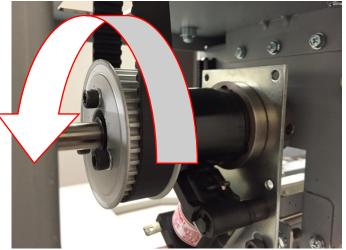
13. Repeat Steps 10 to 13 until the Punch shaft flats are horizontal. It is important to turn the punch shaft with a wrench until it hits a hard stop in the counter-clockwise direction (viewed from rear side). Important note: Turning the shaft with hand will not provide enough torque and the setting will be incorrect. Therefore use a wrench to turn the shaft.
