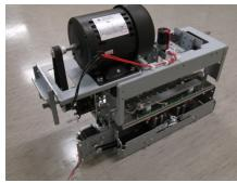
4. Remove the left or right Die Lock Bracket Screws (2).
