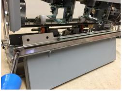
11. Remove Nuts (3) and the Chip Chute.
