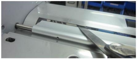
The clearance should be minimum 1.0 mm.
