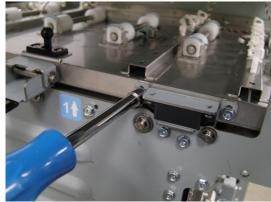
8. Remove the Handle assembly by removing (2) screws.
