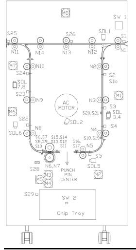
If the Punch is enabled, the transport and punch motors are started, and the Divert Solenoid SOL 1 is activated to direct the sheets into the punch path.
