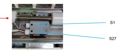
2. Make sure the sensor wire is connected securely at the Sensor and at the Main Control Board. Do ARP 1.6 to remove the Rear Cover to gain access to the connector at the Control Board.
