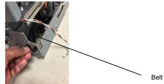
7. Disconnect the Left/Right Steering Stepper Connectors at the Punch Frame. One of the Connectors has 6 pins the other has 7 pins.
