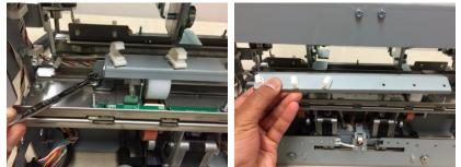
6. Unplug the Alignment Sensor Connector
