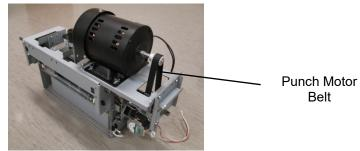
4. Do ARP 3.6 Punch Motor Belt Replacement (Timing Belt) to remove the Punch Motor Belt.
