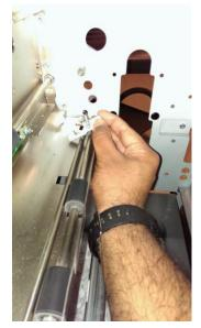
11. Remove Accel Panel Rear and Front Latch assemblies to remove the Accel Idler Latch shaft.
