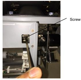
8. Remove the Socket Head Cap Screw and Split Lock Washer from the Cam and the Shaft at the front of the Punch Module.
