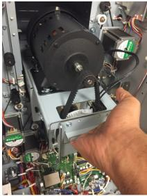
• Reach in and grasp the rear handle and continue to slide the punch. Lift the punch off the rail- DO NOT let it drop on the control board.
