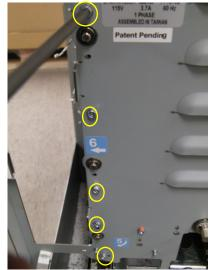
10. Remove (5) screws from the rear frame that mount the Exit drive panel.
