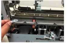
8. Transfer the Skew Sensor, Steering Idler Roller, Idler roller Cover, and all fasteners to the new Weldment.
