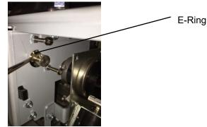
10. Remove the E-Ring from the Shaft at the front of the Punch Module.
