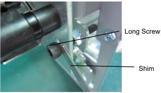
8. Use a 10 mm wrench and a 6mm Allen Wrench to tighten the Lock Nuts (2).
