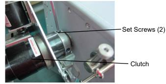
You can press down on the actuator and turn the punch shaft to orient the set screw in any direction for easy access.
