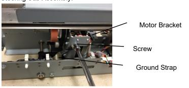
6. Remove the Phillips Screw and Nut from the Ground Strap at the Alignment Carriage Sub Assembly.
