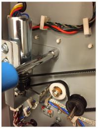
7. Remove the Diverter Solenoid Sub-assembly.
