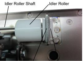
Retaining Spring Bearing Housing
