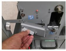
7. Do ARP 2.27 to remove Motor M7 by removing (4) screws.
