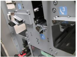
3. Loosen the Nut and Lock Screw.
