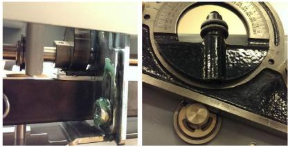
7. To index the shaft to the correct position, remove the spring clip from the its groove in the Punch clutch.
