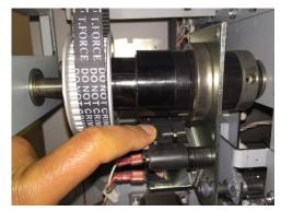
8. Remove the Clutch from the Shaft.
