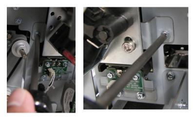
• Rotate the Clutch along with the shaft in the opposite direction (clockwise CW direction when viewed from the back) until the pins exit the sheet.
