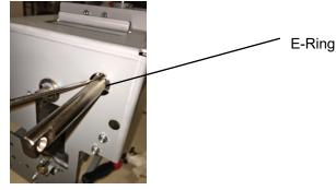
11. Pull the Shaft out through the Cams (2) and out of the Punch Module.
