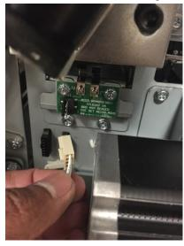
15. Disconnect the Connector for Sensors S16 and S17.
