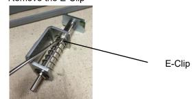
• Pull the Die Lock Plunger and Stripper out.
