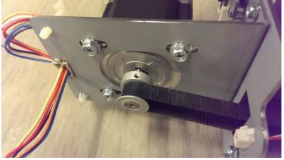
The set screws are secured tightly. Yes- Escalate to higher level No- Tighten set screw(s) and return to normal operation
