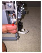
• Press down on the top tab to remove it from the top side. Then press the bottom tab to release the connector fully.
