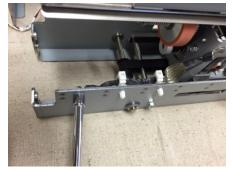
7. Remove the Ground Strap from the Wire Saddles.
