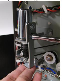
NOTE: Raising the Limiter Bracket too high will position the diverter gate higher, which will obstruct the paper flow and cause jams.
