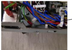
5. Remove the M4 Screws (4) from the side of the Base Frame.
