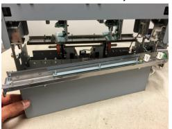
9. Die rail springs can be replaced at this point by unscrewing M2 screws (4) and M2 lockwashers (4). If you are replacing only the springs, go to Installation procedure.
