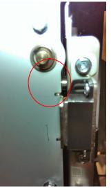
When the idler panel is opened and closed, you should be able to see 3. the Idler springs extend, which will ensure proper idler roller pressure.
