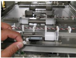
5. Remove the screw and nut for the ground strap.
