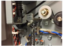
5. Disconnect the inline Connector for the Diverter Solenoid subassembly. 6. Remove Screws (2) from the diverter solenoid sub assembly.
