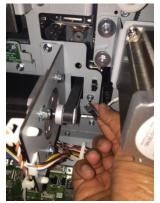
11. Disconnect the Connector for Solenoid SOL2.
