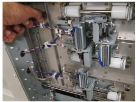
6. Disconnect the Connectors for Sensors S22, S23, & S24 at the sensor
