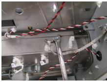
5. Open the Cable Clamps to release the Sensor Cable.
