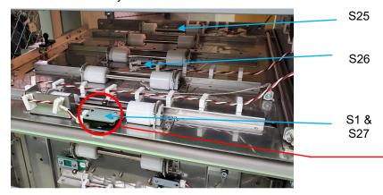
Sensors S1, S25, S26, and S27 are on the Upper Bypass Panel (PL 3.5).
