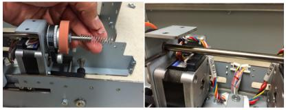
7. Remove the drive roller shaft and all the components on the drive shaft. (4 plastic washers; 2 springs; 2 drive rollers; 2 belts; 4 e-clips)
