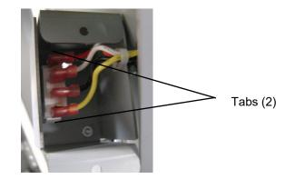
6. Note the location of the Wires (4); then disconnect the Wires from the Interlock Switch (PL 1.2).
