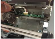
8. Disconnect the Alignment sensor board connector.
