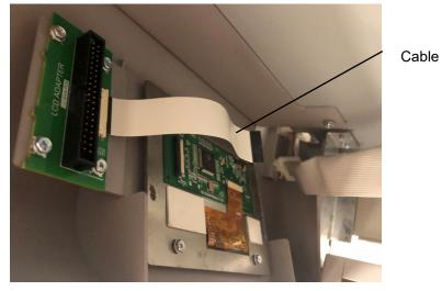
5. From the bottom side of the Top Cover, remove the Screws (4) holding the LCD Display to the Top Cover.
