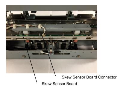
5. Remove the Nuts (4), Washers (4), and the Skew Sensor Board. (do not remove the washers under the sensor board)
