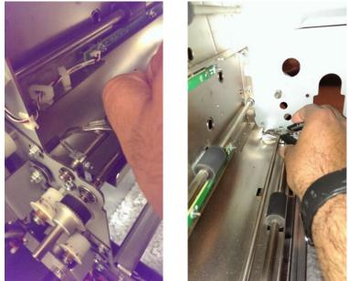
5. Remove the M3 screws (2) from the Accel Idler Panel Front and Rear Latches.
