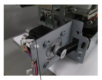
Punch Alignment Stepper Motor (M5)
