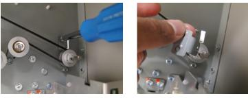
10. Remove the Upper Bypass Assembly.
