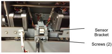
5. Remove the Sensor Sub-assembly.
