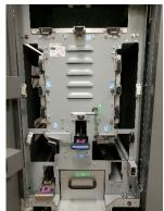
3. Remove the two screws [1] on the Door Latch.
