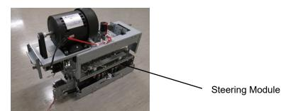
5. Remove the Steering Idler and Drive Panel assemblies by removing the M3 Nuts (4)
