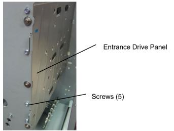
12. Remove the Screws (5) that hold the Entrance Drive Panel to the Rear Frame.
