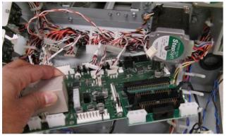
6. Disconnect the plug-in Connector and remove the Comm Board.
