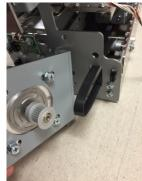
6. Pull the Alignment stepper belt in through the hole in the Frame.
