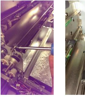
6. Remove the E-clip from the Accel Idler Shaft on the rear side.
