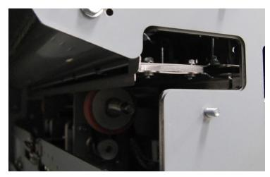
5. Check that the Steering Drive (Drive Panel Steering Sub Assembly) and the Idler Panels should be centered to the guide brackets as shown.
