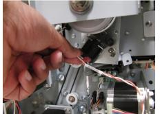
Remove two screws that hold the Punch Clutch Bracket
