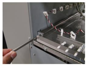
7. Remove (2) Idler panel magnetic latches from the Upper bypass assembly by unscrewing (4) screws.
