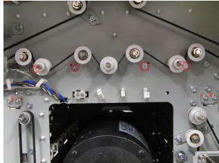
2. Using the Reference holes in the front/rear frame (4 holes in the front frame and 4 holes in the rear frame) and the sheet metal panel, position the drive panel to ensure the drive rollers protrude 1.5±0.5mm through the drive panel.
