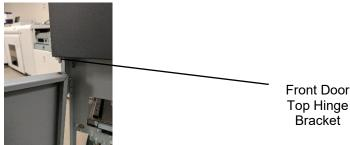
4. Remove the Screws (2) and the Front Door Top Hinge Bracket on the inside of the machine
