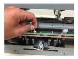
5. Remove the Screws (4) that hold the Steering Idler Panel Sub Assembly to the Drive Panel Steering Sub Assembly.
