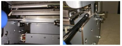
8. Remove both upper and lower brackets as shown, do not pull on the Align sensor wires.
