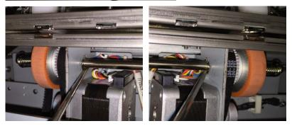
6. Remove the Shaft from the Drive Panel Steering Sub Assembly.
