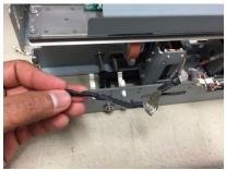
8. Remove the Steering Carriage Ground Strap.
