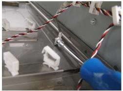
6. Remove (2) E-clips from the hinge shaft and remove the shaft.
