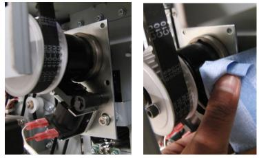
4. Inspect the collar stop and the metal insert pawl for any wear.
