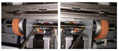
5. Slide the Shaft in the opposite direction so that the Steering Drive Roller Spring, (2) plastic washers and Steering Drive Roller can be removed (from the side that needs the part replaced).
