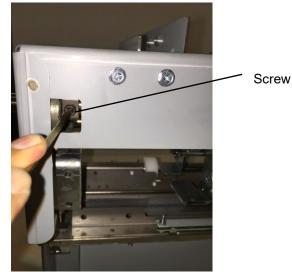
9. Remove the E-Ring from the Shaft at the rear of the Punch Module.
