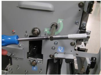
7. Remove the M4 Screws (5) from the Front Frame. The screws to be removed are marked with a downward arrow (★).
