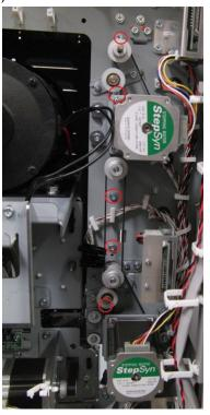
2. Using the Reference holes in the front/rear frame (4 holes in the front frame and 4 holes in the rear frame) and the sheet metal panel, position the drive panel to ensure the drive rollers protrude 1.5±0.5mm through the drive panel.
