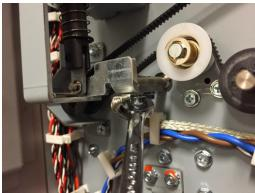
5. Remove the E-clip from the Diverter Shaft on the rear side.
