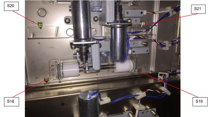
Sensors S18 and S19 are on Mid Punch Large Backgage Sensor Board. Sensors S20 and S21 are on Mid Punch XL Backgage Sensor Board.
