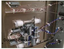
5. Disconnect the Connectors for Sensors S2, S3, & S4.
