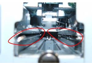
3. Remove the M4 Nuts (3) and the cover for Area 5.
