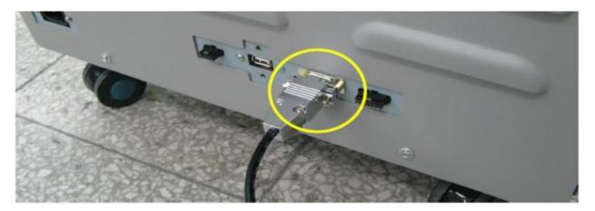
c) Replace the finisher rear maintenance cover. Ensure that the communication cables are not pinched anywhere.
