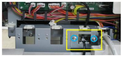
b) Plug the free end of the communication cable to the communication port of the SmartPunch Plus in the rear side of the machine.
