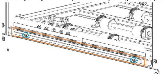
Attach exit upper guide with the supplied M4-8mm long round tipped screws
