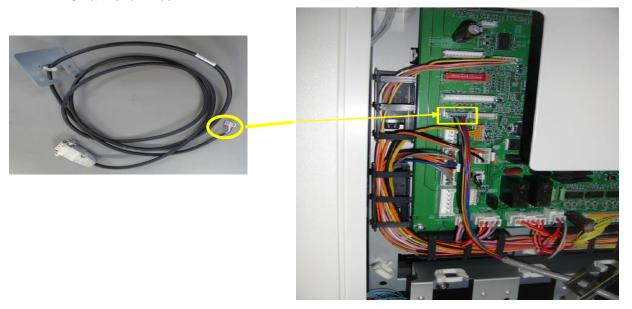
ii) Attach the bracket tied to the communication cable with the supplied M4-8mm long round tipped screws (2 places).
