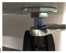
Using the 17mm (11/16") wrench, rotate the caster stems to change the height.
