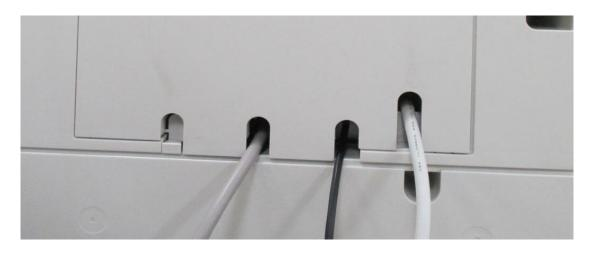
d) Connect the supplied AC power cable to the SmartPunch Plus on the rear side lower left corner. SmartPunch Plus has a power switch on the front of the machine. Ensure this is turned on.
