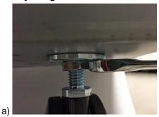
Using a 19mm (3/4") open ended wrench, loosen the jam nut(s) situated on the caster stud under the base of the machine.
