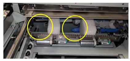
21. Place the spare magnet strips from the installation kit on the element feeder as shown below. When storing them on the element feeder, ensure that they are completely on the flat face of the drawer and are not near the spool.
