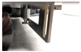
11. Using the M5 screws provided, secure the bracket to the eWire base. The mounting holes on the eWire base are slotted and the brackets location can be adjusted. Refer to the install manual of the downstream device for the positioning of this bracket.
