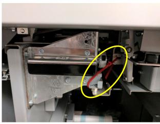
18. Remove the zip ties securing the closer module the side frame of the eWire.
