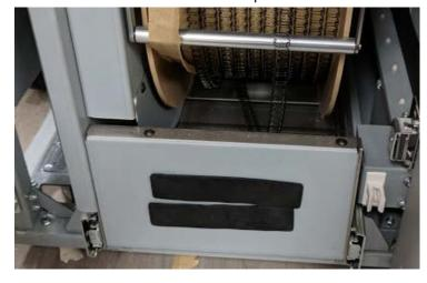
22. Take the wire cutters from the installation kit and install them into the triangular pocket located behind the element feeder door. Place the Element Height Setup Tool and the Punched Hole Position check tool on the inside of the book drawer as shown below. Secure the Element Height Setup Tool using the M4 screw provided.
