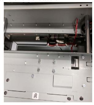
20. Remove the foam shipping blocks from the front and rear that keeping the holder in place.
