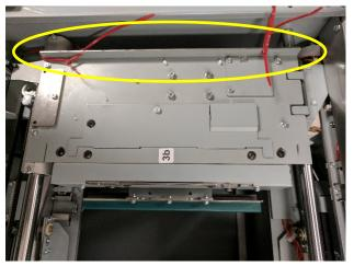
19. Move the closer module by hand to reveal the cable tie on the holder frame. Remove the cable tie.
