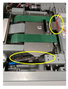
17. Remove the zip tie from the Drawer Lockout mechanism where shown.
